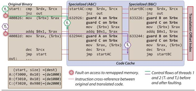
Figure 8. Control transfer on access fault from original binary, to specialized blocks in the code cache
